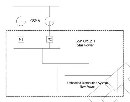
In this example, there are two Distribution Systems and two LDSOs in GSP Group 1. Star Power is the Nominated LDSO (i.e. ex-Public Distribution System Operator) for GSP Group 1 and New Power is an embedded LDSO).
