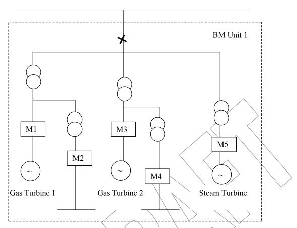
This example comprises of two gas fired turbines and one steam turbine connected to the Transmission System. The equipment is owned and operated by Star Power. The equipment cannot be independently operated and therefore Star Power has registered them as one BM Unit.
