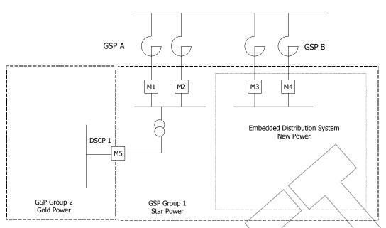
In this example, there are two Distribution Systems in GSP Group 1. Star Power is the Nominated LDSO for GSP Group 1 and New Power is an embedded LDSO. There is a DSCP to GSP Group 2 where Gold Power is the Nominated LDSO. It should be noted that the <u>Aaggregation Reules</u> for GSP Group Metered Volumes would not change if the two GSPs A and B were physically distinct, as they are in the above diagram, or connected.
