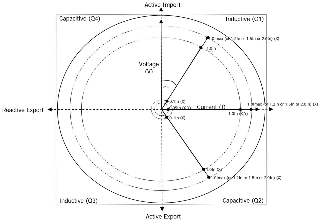
**Figure 1: Example showing Type A Calibration Points for a CoP1 and 2 Reactive Energy Meter**
